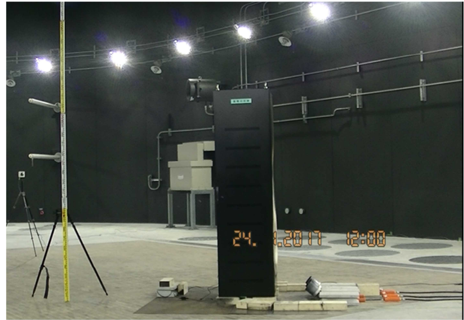
Fig. 8 Rack image after 90-minutes burning (Gas valves shut off)
