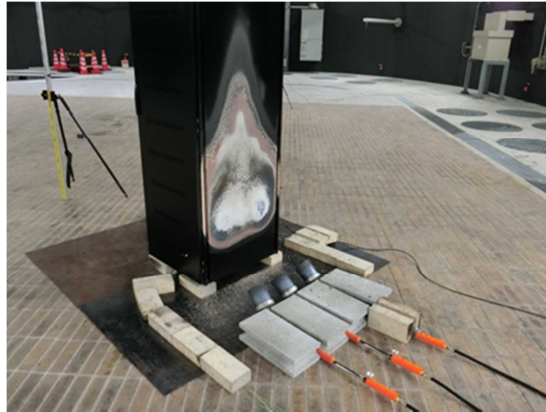
Fig. 12 Sample surface after fire exposure
